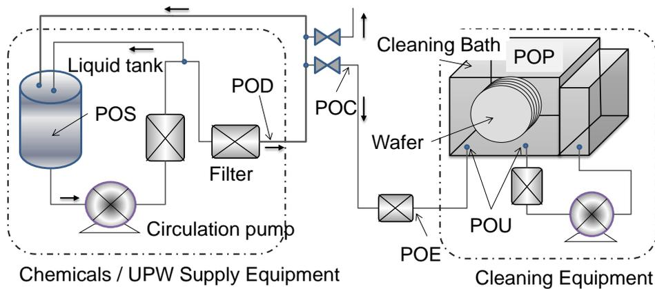
Fig. 1 Particle measurement points in the wet process.
