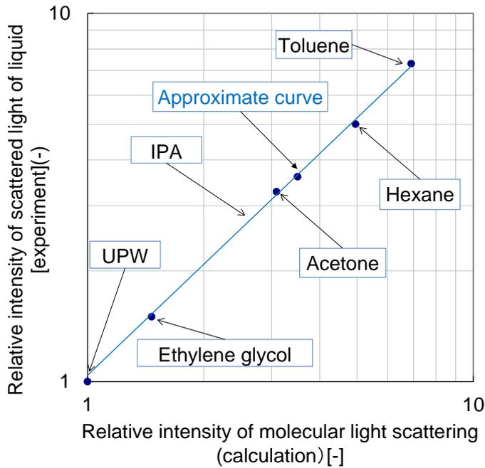
Fig. 8: Light scattering in liquid received by the particle detection system of LPC.
