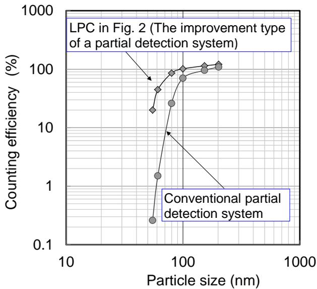
Fig. 4 Evaluation of particle counter performance by a quantitative dilution method.
