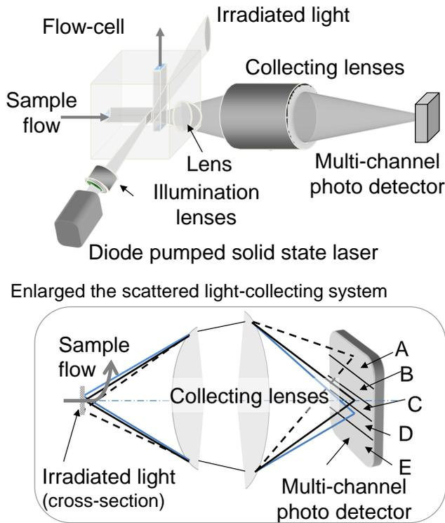
Fig. 2: Particle detection part of the 40nm compatible liquid-borne particle counter.
