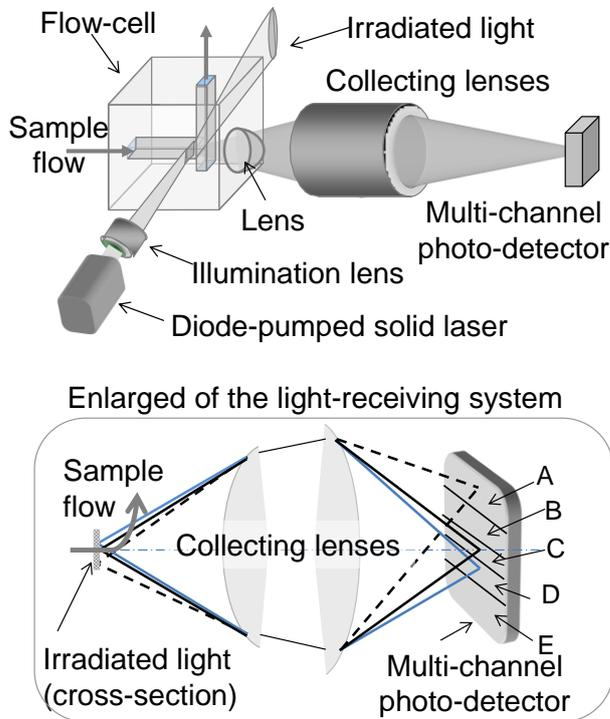
Fig.3 Particle detection system of liquid-borne
