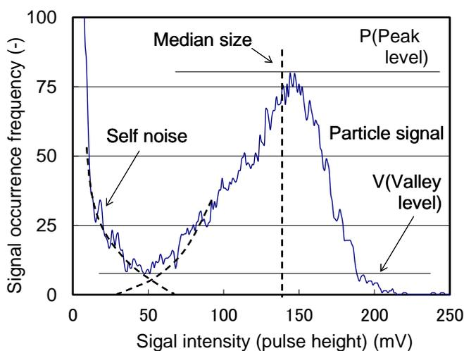
Fig. 4 Pulse height distribution for test particle-sensing signals.
