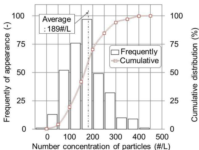
Fig. 7 Measurement of particles in UPW using liquid-borne particle counter for 50 nm.
