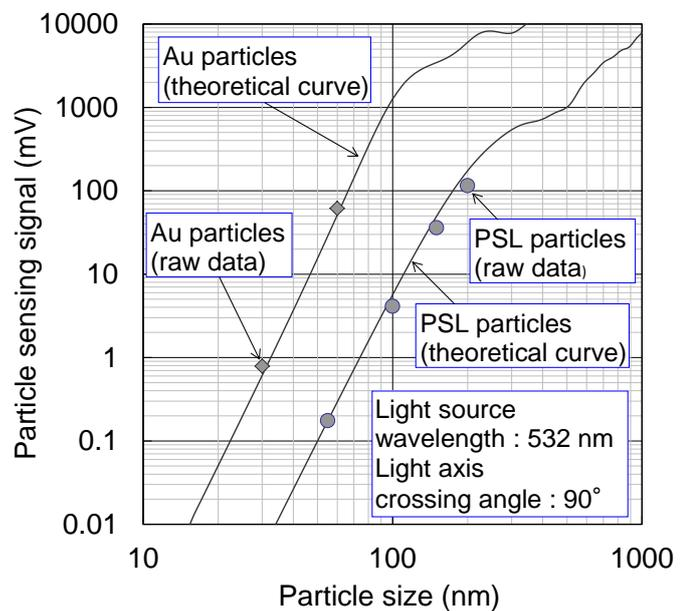
Fig. 9 Light-scattering characteristics of PSL particles and Au colloidal particles
