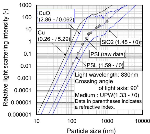
Fig.1 Light-scattering characteristics of particles, derived from Mie's light-scattering theory.
