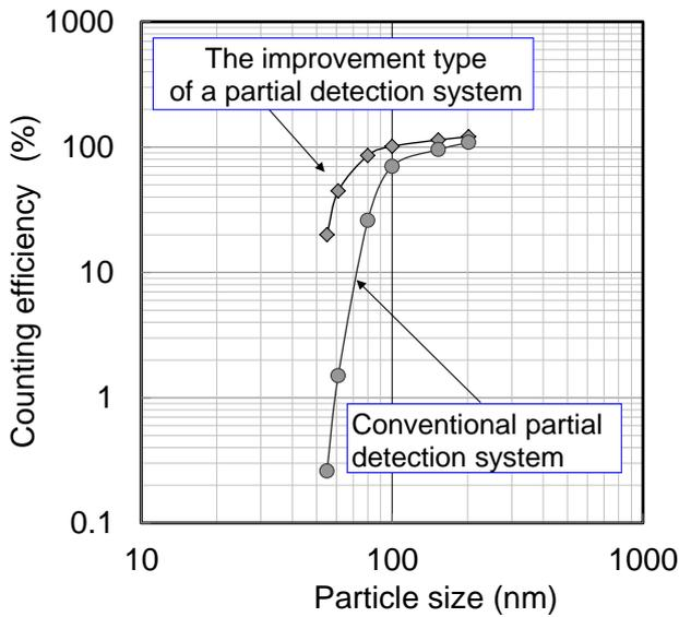
Fig. 6 Evaluation of particle counter performance by a quantitative dilution technique.
