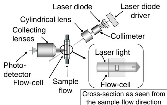
Fig. 2 Particle detection part of liquid-borne particle counter for 200nm.
