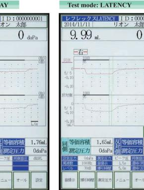
Measure with posting stimulus tone for 10 seconds at the set frequency and level. Measurement time 12.5 seconds
