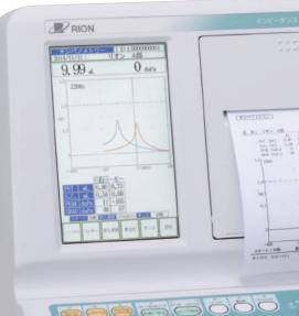
1000 Hz probe tone, can do tympanometry that is suitable for newborns.
