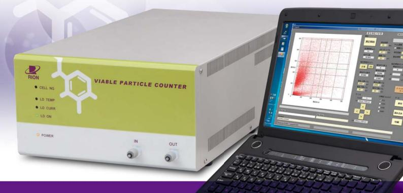
The device incorporates a fluorescence detection function using an ultraviolet laser light source. Reflected light from particles as well as the light emitted by autofluorescent content of the viable particles themselves is utilized to distinguish between non-viable and viable particles for counting.
