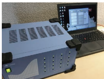
Measuring reverberation time (SA-02M, AS-20PC5)
