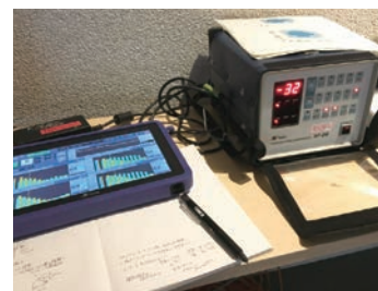
Measuring sound insulation (RIONOTE, SF-06)
