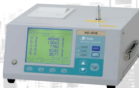
Fig.3. A particle counter of the same model as the one installed inside the AOH (Rion KC-01E)
