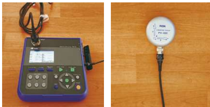
Fig.2. How the vibration level meter VM-55 (left) and vibration sensor (right) are set up
