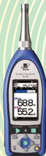
Fig.3. Measurement system Left : RION High-Precision Sound Level Meter NL-62 capable of measuring low frequency sound. “The NL-62 can record waveforms, which significantly reduces the number of instruments needed.” (by Mr. Fukushima) Right : Dual windscreen design.Placing a weight at the base was Mr. Fukushima's idea.
