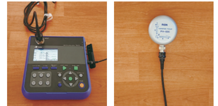
Fig.2. How the vibration level meter VM-55 (left) and vibration sensor (right) are set up The VM-55 allows long-term recording and storing in SD memory cards of vibration levels on three axes (X/Y/Z), 1/3 octave band acceleration levels, and even vibration acceleration waveforms simultaneously.
